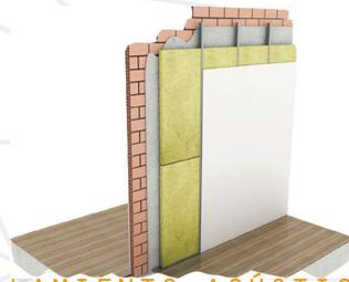
AISLAMIENTO ACÚSTICO EN MUROS
