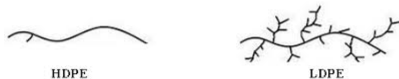
Figure 1: Structure of HDPE and LDPE
