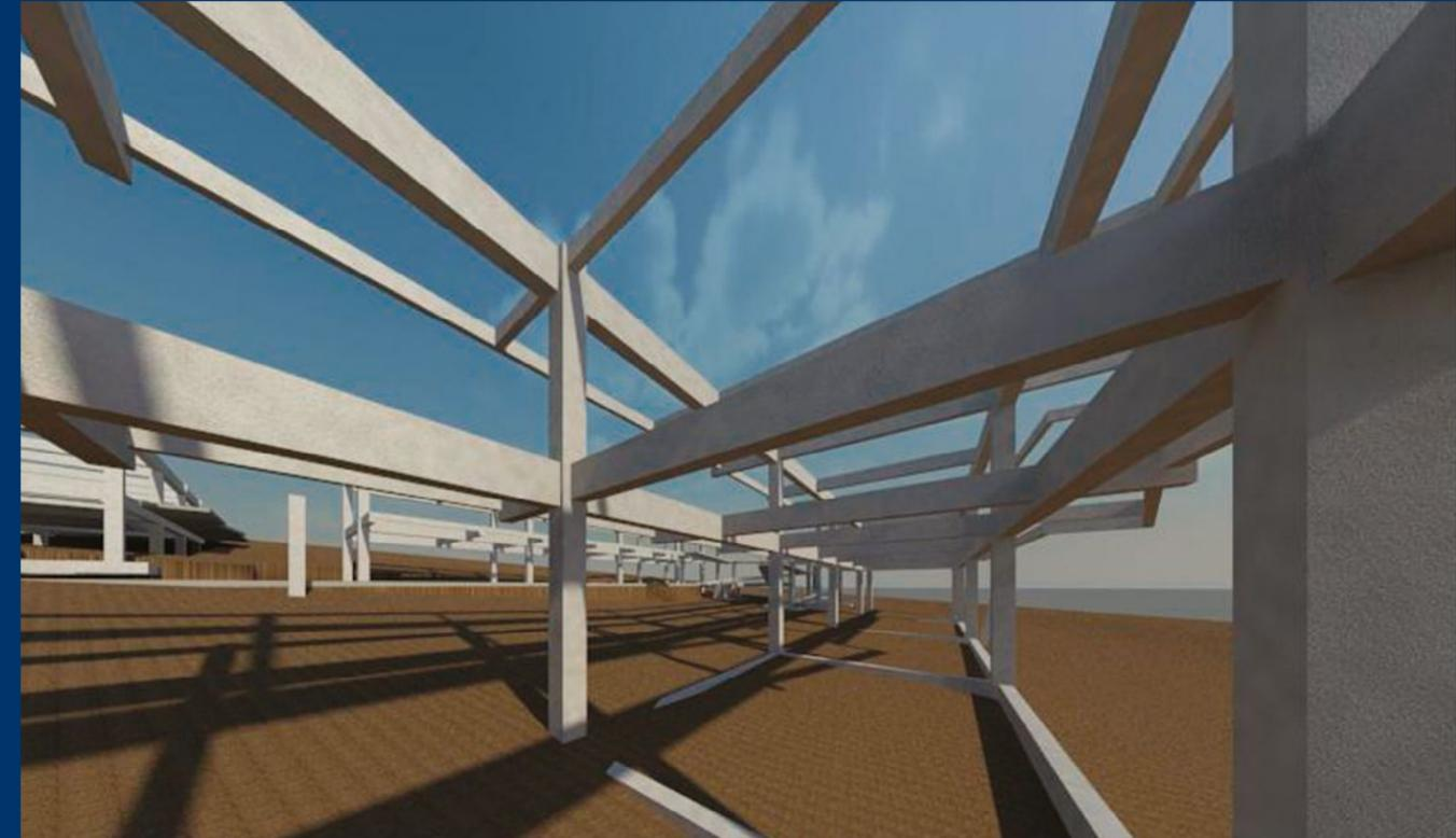
**VISTA ESTRUCTURAL INTERIOR CON COLUMNAS, VIGAS PRINCIPALES, VIGAS SECUNDARIAS Y VIGAS DE REMATE.**
