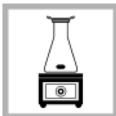
7. Use a watch glass as the flask cover. After the reagents dissolve, increase the temperature of the sample to 90 °C (194 °F). Do not boil. *Note: It is not necessary to increase the temperature for a mercury standard or reagent blank in distilled water.*
