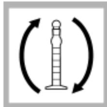
2. Put the stopper on the receiver. Invert to dissolve the reagent.
