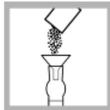
3. Use the supplied funnel to add the contents of one HgEx Reagent 4 foil pillow to the Distilling Receiver.
