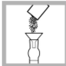
1. Use the supplied funnel to add the contents of one HgEx Reagent 3 foil pillow to the eluate in the Distilling Receiver.
