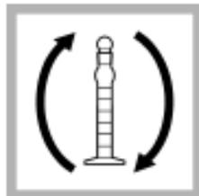
6. Put the stopper on the receiver. Invert to mix the reagent.
