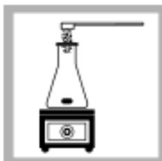
5. Add 4.0 g of potassium persulfate to the sample. Alternatively, add one 5 gram measuring scoop of potassium persulfate to the sample. Stir until dissolved.
