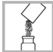
12. Remove the cell from the cell holder. Add the contents of one HgEx Reagent 6 foil pillow to the solution.
