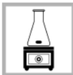
10. Put the cool digested sample on the cool stirring hot plate. Set the stirrer power to on.
