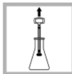
12. Remove the stir bar. The digested sample is now ready for the cold vapor separation and preconcentration procedure.
