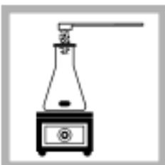
6. Add 7.5 g of potassium permanganate to the sample. Alternatively, add a 10 gram measuring scoop of potassium permanganate to the sample. Stir until dissolved.
