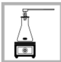
11. Add hydroxylamine-hydrochloride until all manganese dioxide is dissolved. Use a 0.5-g measuring spoon to add 0.5 g additions of hydroxylamine-hydrochloride until the purple color is gone. Wait 30 seconds after each addition and look for the color change.
