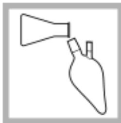
1. Pour the digested sample into the Cold Vapor Gas Washing Bottle.
