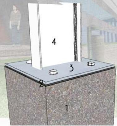
DETALLE DE TRONCO DE COLUMNA FUNDIDO PARA COLUMNAS DE ACERO.
